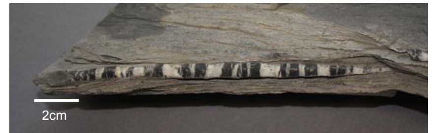
Figure 5: An extended belemnite, an example of positive elongation. The dark areas are the original fossil and white a calcite infill (J. Houghton).
